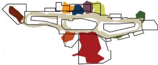
Figure 15: Constructed floor plan of storey 2 by CrowdInside++, which has several artificial improvements that are not always possible in reality.
